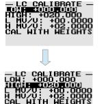
Enter the value in engineering units of the high calibration point of the system eg. 5000kg. This is normally the full rating value of the load cells.
