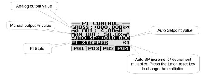
Use the up/down and keypad to adjust the MAN OUT and AUTO SP value.
