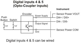
either in a common ground or a common supply configuration
