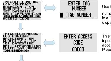
Use the left, right and the alpha-numeric keypad to enter the tag number. Press EACK for a space character. If the first character is a "%" then the date and time will be displayed on the main display instead of the tag number.
