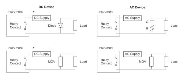
An optional noise suppression device can be ordered. Install these devices as close to the load as possible.
