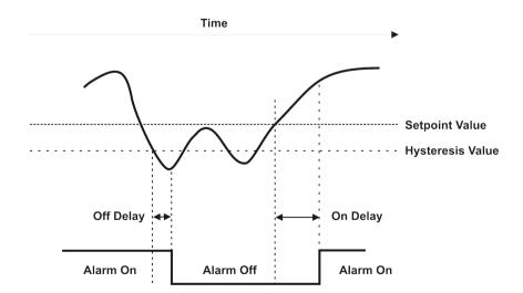
The above diagram illustrates the use of a high alarm with hysteresis and on/off delay.
