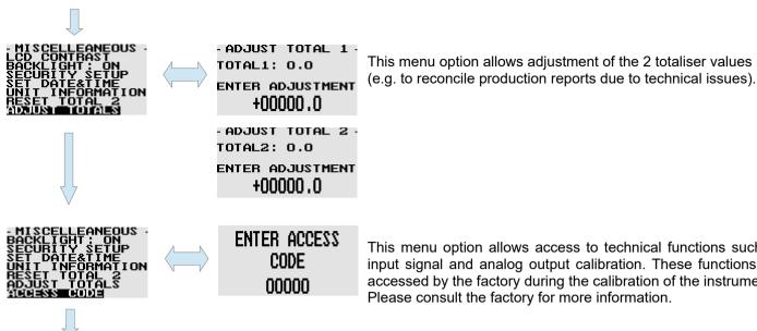
This menu option allows access to technical functions such as input signal and analog output calibration. These functions are accessed by the factory during the calibration of the instrument. Please consult the factory for more information.
