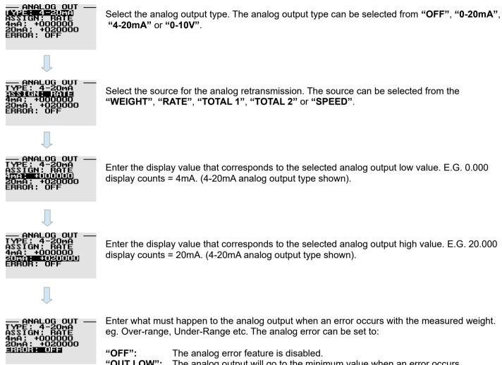
**"OUT LOW":** The analog output will go to the minimum value when an error occurs. **"OUT HIGH":** The analog output will go to the maximum value when an error occurs.
