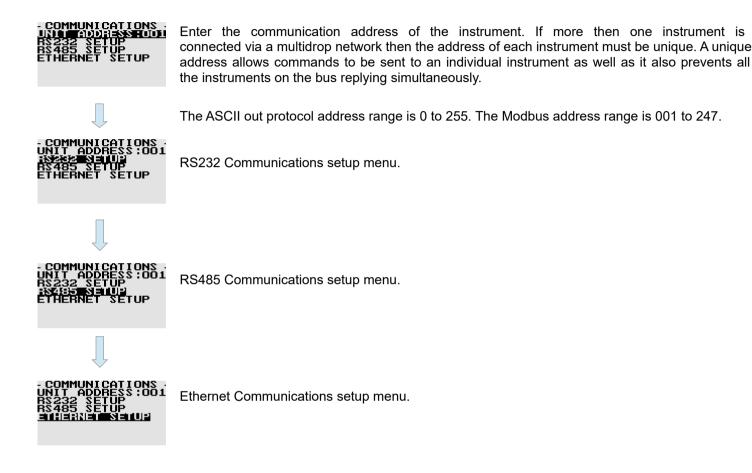
The instrument has 3 built in communication protocols:
