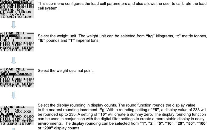
Select the weight unit. The weight unit can be selected from "kg" kilograms, "t" metric tonnes, "Ib" pounds and "T" imperial tons.
