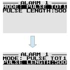
Enter the pulse width in milliseconds of the output pulse.
