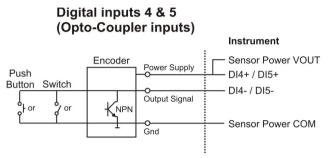
Digital inputs 4 & 5 can be wired either in a common ground or a common supply configuration
