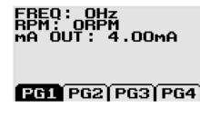
This display page shows the following parameters: Rate, Totaliser 1 (resettable totaliser), Totaliser 2 (non-resettable totaliser), Speed, Belt Load (Weight) and the Tare value. Pressing the PG1 key again will display extended information such as frequency, RPM and the analog out value.
