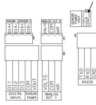
Select +12Vdc or +24Vdc Sensor Power
