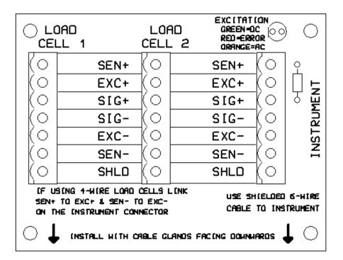
Note: Install with cable glands facing downwards and with cable drip loops
