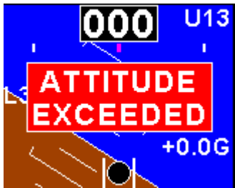
Message displayed when the maximum bank, pitch or yaw rates have been exceeded
