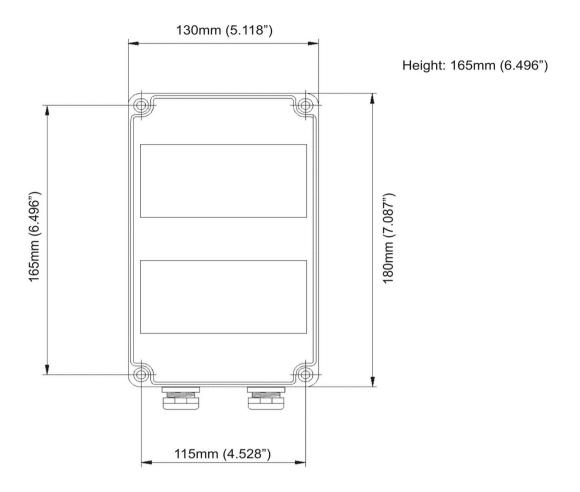
The 2<sup>nd</sup> panel meter can be installed by simply clipping the blanking plate away with a side cutter.
